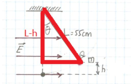
First we note that the system is in equilibrium. This means that the sum of the forces in both the  $x$  and the  $y$  directions are equal to zero. We will use this fact (and some trigonometry) to obtain the height the bob gets displaced.
